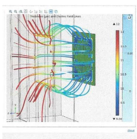
This graphic is not a detailed example of a smart cathode shield but it does point out the basic difficulty in electroplating flat cathode panels with uniform metal deposit thickness. Shield construction ensues using a pattern suggested by evaluating the plating thickness uniformity on the panel and affixing a non-conductive barrier to the rack, so positioned between the anode and cathode that average current density across the panel surface is made more uniform.
