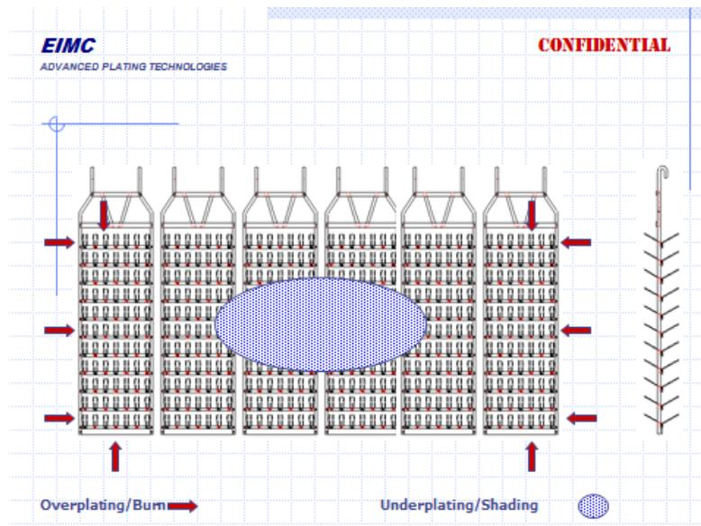
A little trial and error by imposing simple shields or barriers can fix a situation like the one above. All the available plating current still goes into the cell, it's simply redirected. "Shading" begins to go away.
