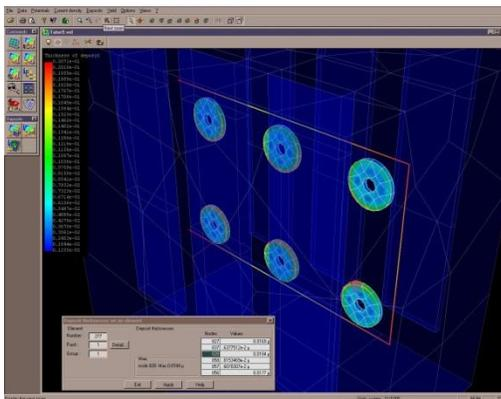
There's a plating shield in this graphic representation of a plating model. It's not real easy to see. The point is that it's not necessary to use a computer model to make a smart plating shield that will benefit the user. A little trial and error can produce significantly better plating results in terms of plating thickness uniformity on a plating rack.
