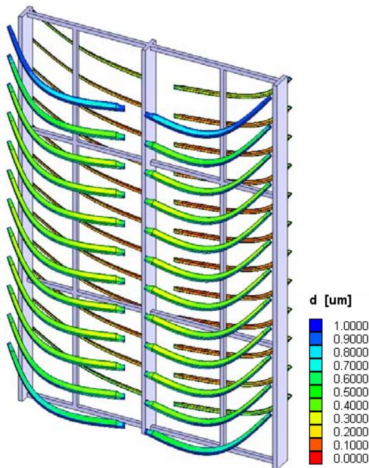
The results of an analysis above illustrate the poor distribution of chromium thickness on a 'standard' rack of trunk finishers. Elsyca solved this customer issue with a modified rack design making appropriate use of shielding and current thieves.
